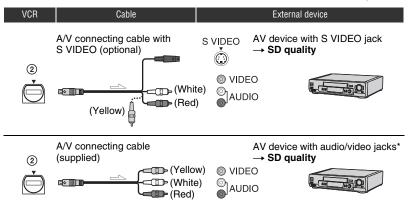
\* When connecting the VCR to a monaural device, connect the yellow plug of the A/V connecting cable to the video jack on the device, then connect the white (left channel) or red (right channel) plug to the audio jack on the device.
